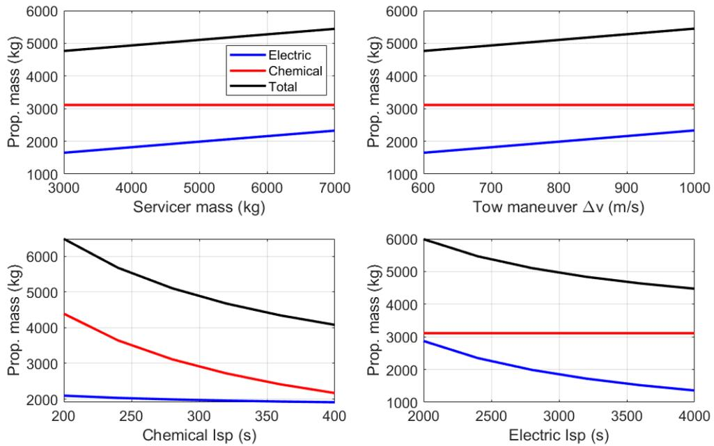
Figure 13: Propellant mass sensitivities to design variables.
