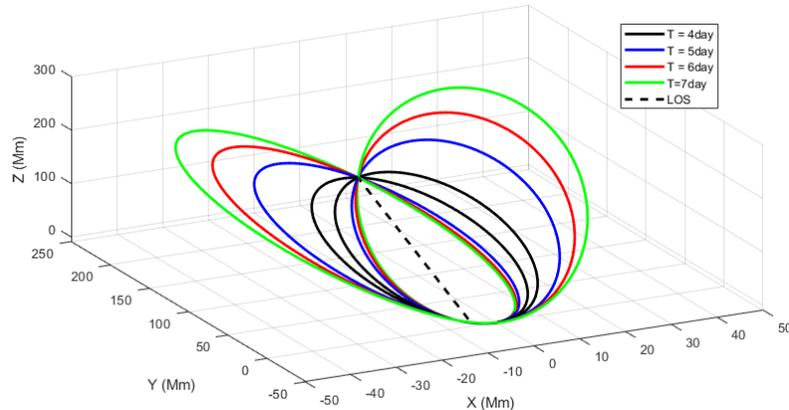
Figure 6: Illustration of orbits with periods from 4-7 days that provide proper alignment with a reference target with a right ascension of 90deg and a declination of 45deg for a nominal separation of 200Mm between the starshade and telescope.
