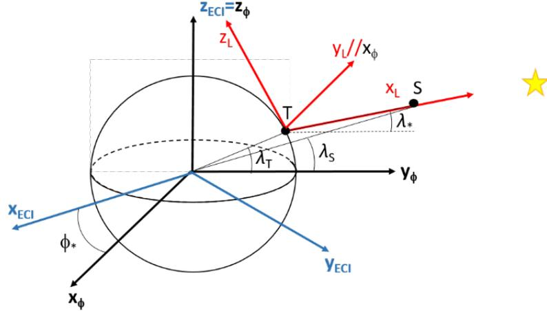
Figure 7: Visualization of coordinate frames including Earth-Centered Inertial (blue, ECI) frame, line-of-sight (red,  $L$ ) frame, and frame aligned with longitude of telescope/starshade/target star (black,  $\phi$ ). S and T stand for starshade spacecraft and telescope.
