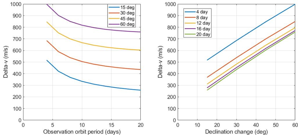
Figure 12: Delta-v cost of up reconfiguration vs angular separation and observation orbit period.
