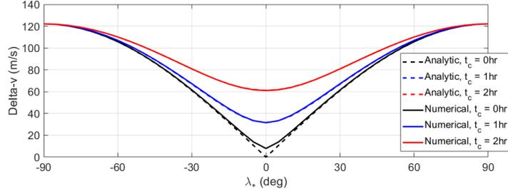
Figure 8: Analytic and numerical delta-v cost of 1hr observation for telescope on equator vs target declination for selected  $t_c$ .
