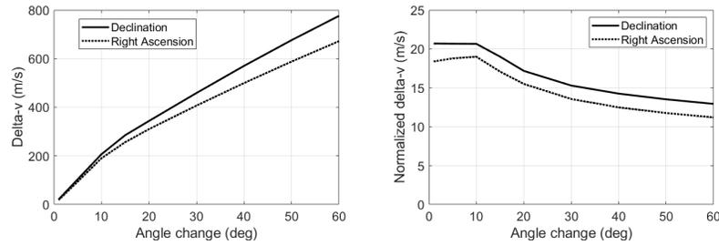
Figure 11: Reconfiguration delta-v vs angular separation (left) and delta-v cost per degree vs angular separation (right).
