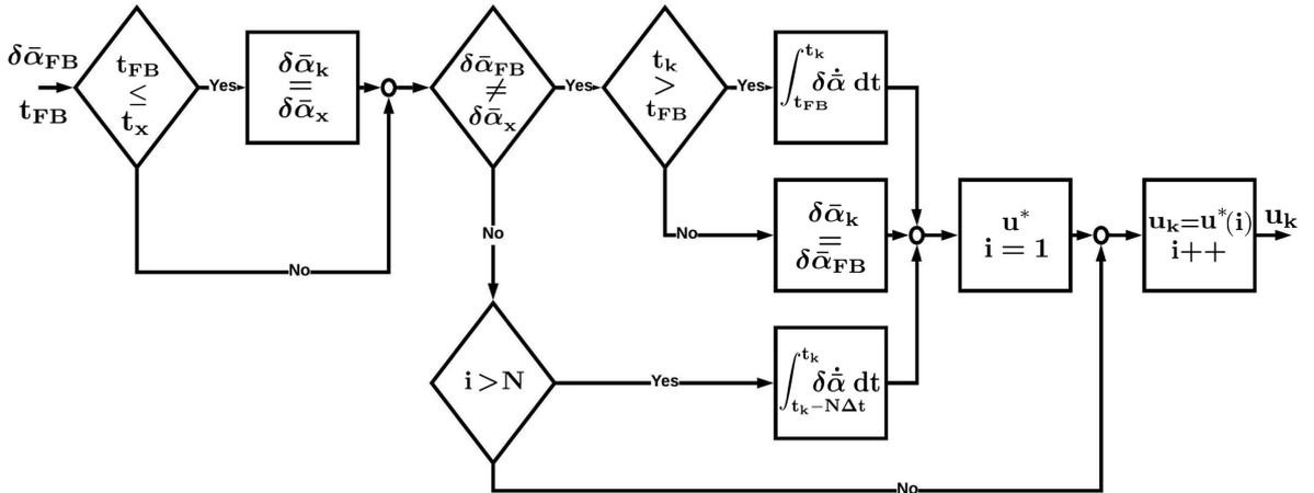
Figure 2. Block diagram representation of the delays/losses compensation structure.
