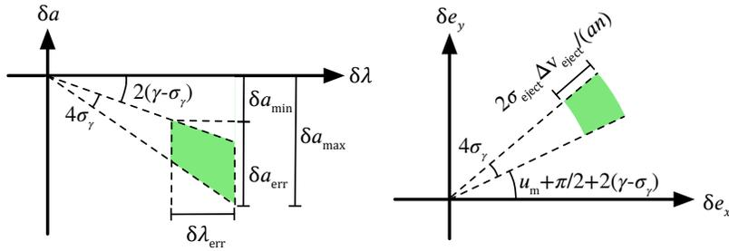
**Figure 4. Possible ROE immediately after ejection including errors.**
