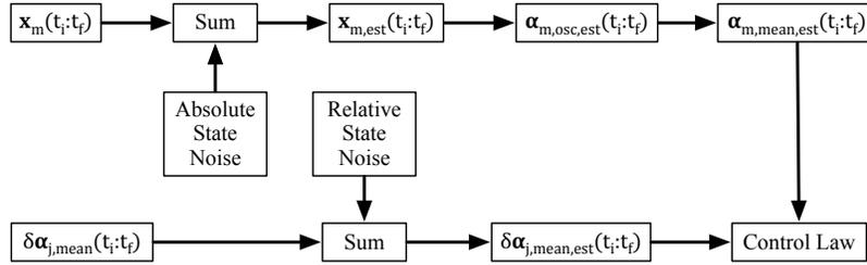
**Figure 9. Computation sequence for thrust commands.**
