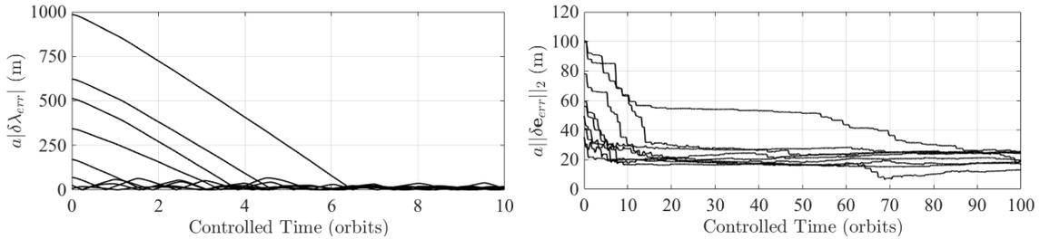
**Figure 11. Time history of  $|\delta\lambda_{err}|$  (left) and  $\|\delta e_{err}\|_2$  (right) for each deputy during forced motion control phase for in-plane formation simulation.**
