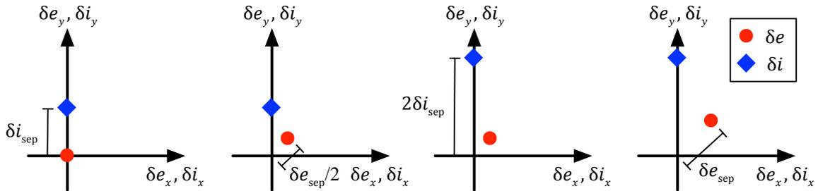
**Figure 6. Evolution of relative eccentricity and inclination vectors of a deployed deputy in an e/i vector separation formation after ejection (left), after the first flight direction maneuver (middle left), after the cross-track maneuver (middle right) and after the second flight direction maneuver (right).**
