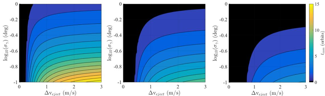
**Figure 5. Maximum allowable commissioning phase duration as function of  $\sigma_\gamma$  and  $\Delta v_{eject}$  for a swarms of 6 (left), 9 (middle), and 12 (right) deputies.**
