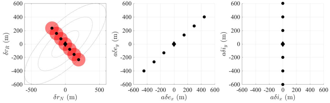
**Figure 2. Example e/i vector separation swarm formation including relative motion in the RN-plane (left) and ROE (middle and right). Regions with insufficient separation from at least one spacecraft ( $< 100$  m) are shown in red.**
