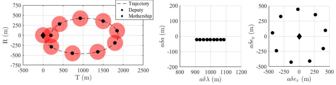
**Figure 3. RT-plane trajectory (left) and ROE (right) for in-plane formation after ejection from mothership. Regions with insufficient separation from at least one spacecraft ( $< 200$  m) are shown in red.**
