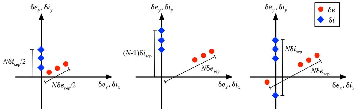
**Figure 7. ROE after deployment of first half of deputies (left), after intermediate maneuver sequence (middle), and after deployment of first deputy from second set (right) in two-sided deployment sequence.**
