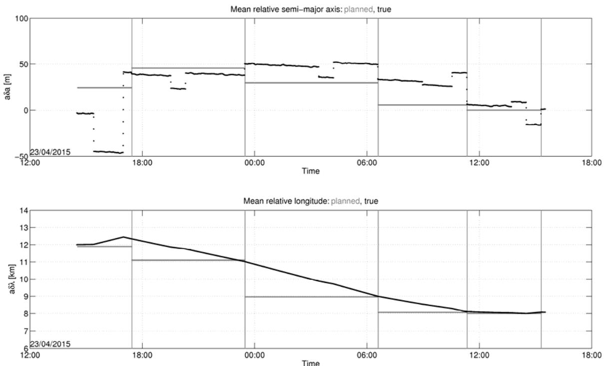
Fig. 11. Control accuracy: true (black) relative semi-major axis (top) and mean longitude (bottom) versus the stepwise planned values (gray).
