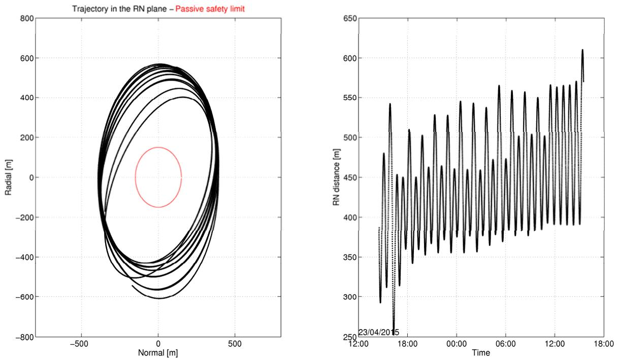
Fig. 15. Passive safety: relative trajectory and minimum distance to the client in the R-N plane.
