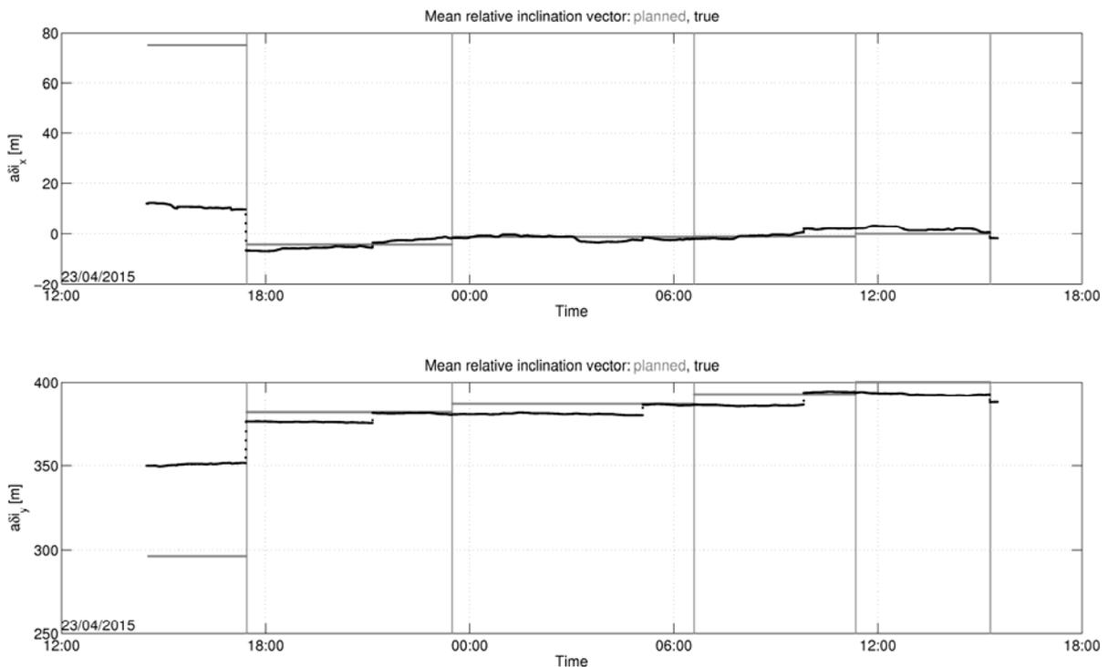
**Fig. 13.** Control accuracy: true (black) relative inclination vector components versus the stepwise planned values (gray).
