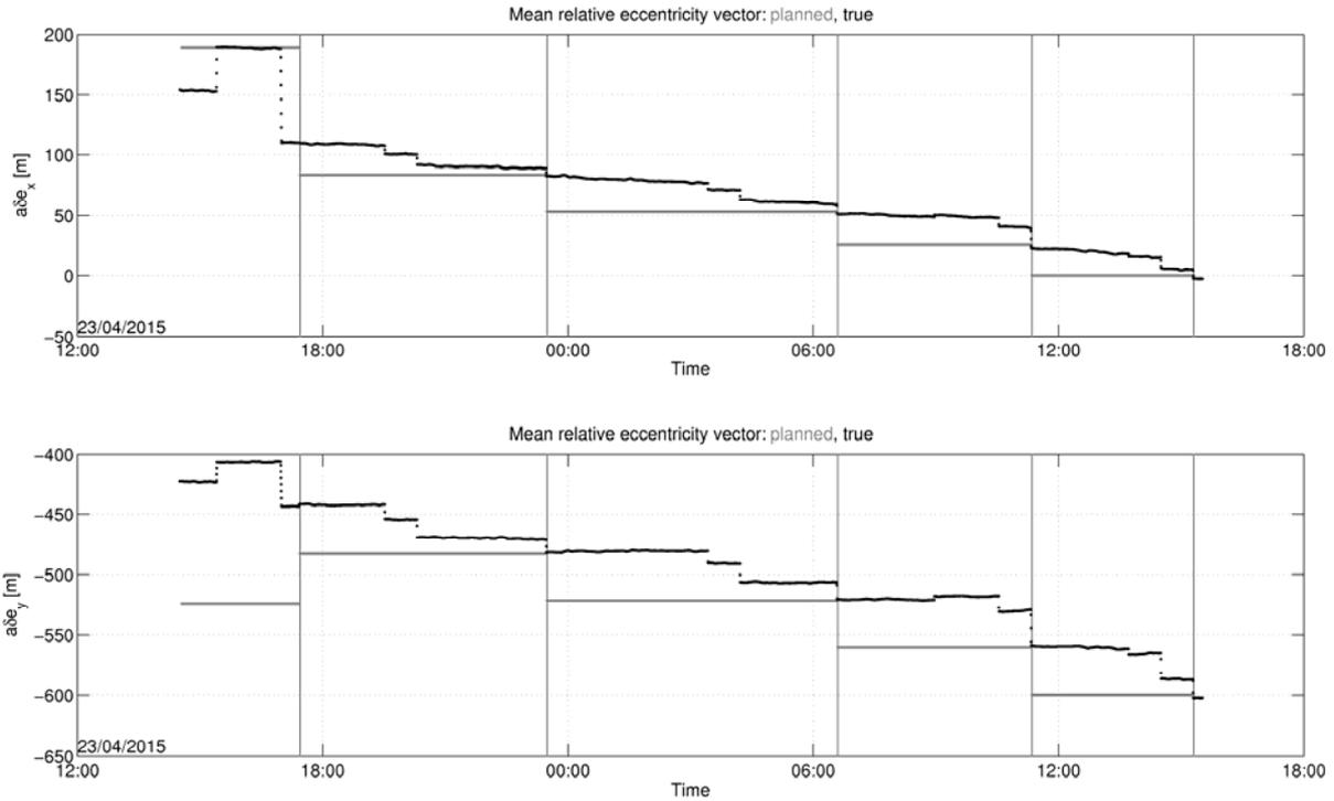
**Fig. 12.** Control accuracy: true (black) relative eccentricity vector components versus the stepwise planned values (gray).
