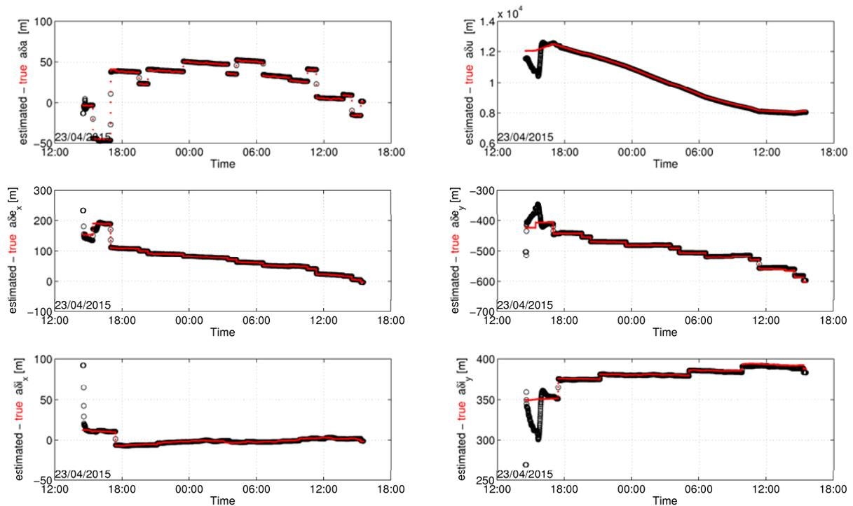
Fig. 8. ROD results: estimated versus true trends of each component of the ROE state.
