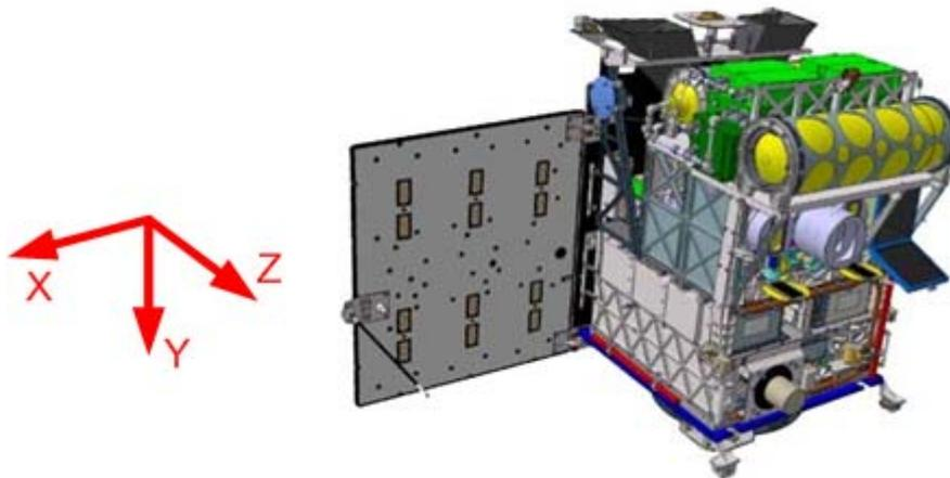
*Fig. 1. The BIROS spacecraft: components view and main orientations with respect to the body frame.*
