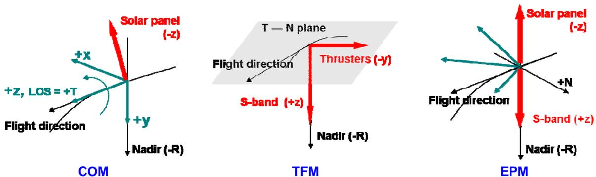
Fig. 2. Attitude modes foreseen during AVANTI: Client Observation Mode (COM), Thruster Firing Mode (TFM), and Earth Pointing Mode (EPM). The local orbital frame (i.e., RTN) is depicted in black, whereas the spacecraft-fixed and camera-fixed frames are respectively marked in red and green.
