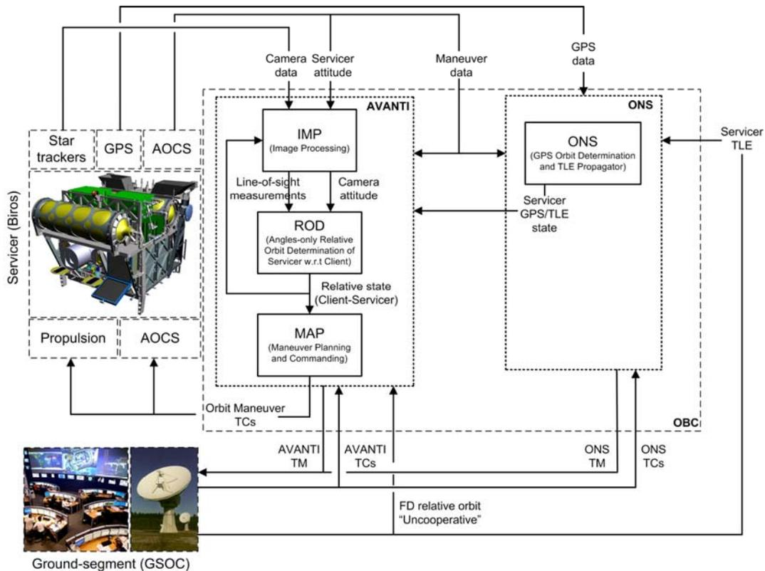
Fig. 3. AVANTI SW architecture and interfaces to space and ground segments.
